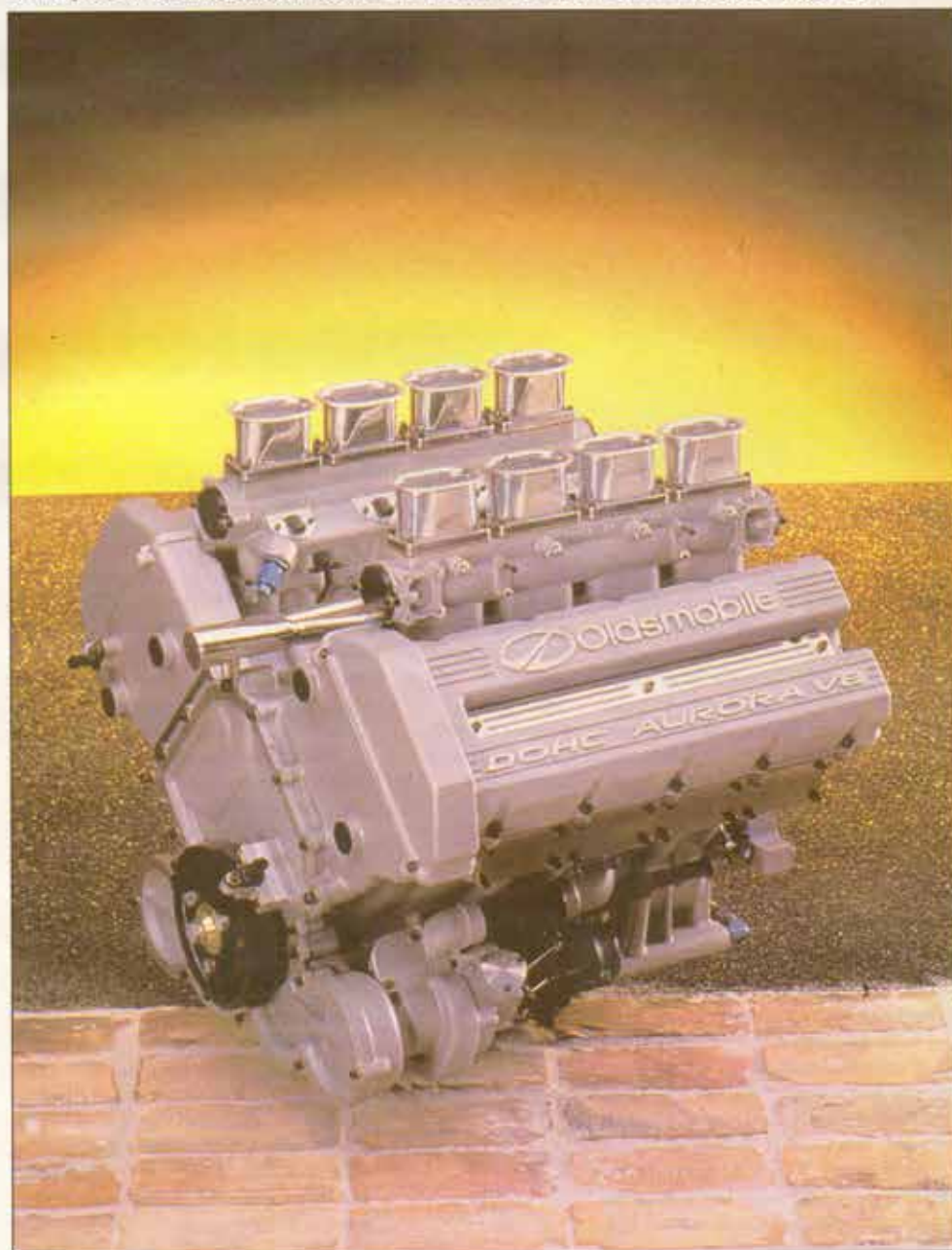
Aurora at the Brickyard: A methanol burning version of Oldsmobile's Daytona winning 4-litre V8 will be built for the 1997 Indy Racing League in the first major commitment by an American automobile manufacturer.
