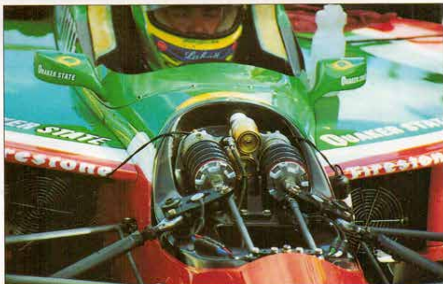
Top: Adjusting the Ohlins dampers in the three-spring front suspension of the 1999 Swift. Above: The Ohlins are a tight fit on the Swift ChampCar.
