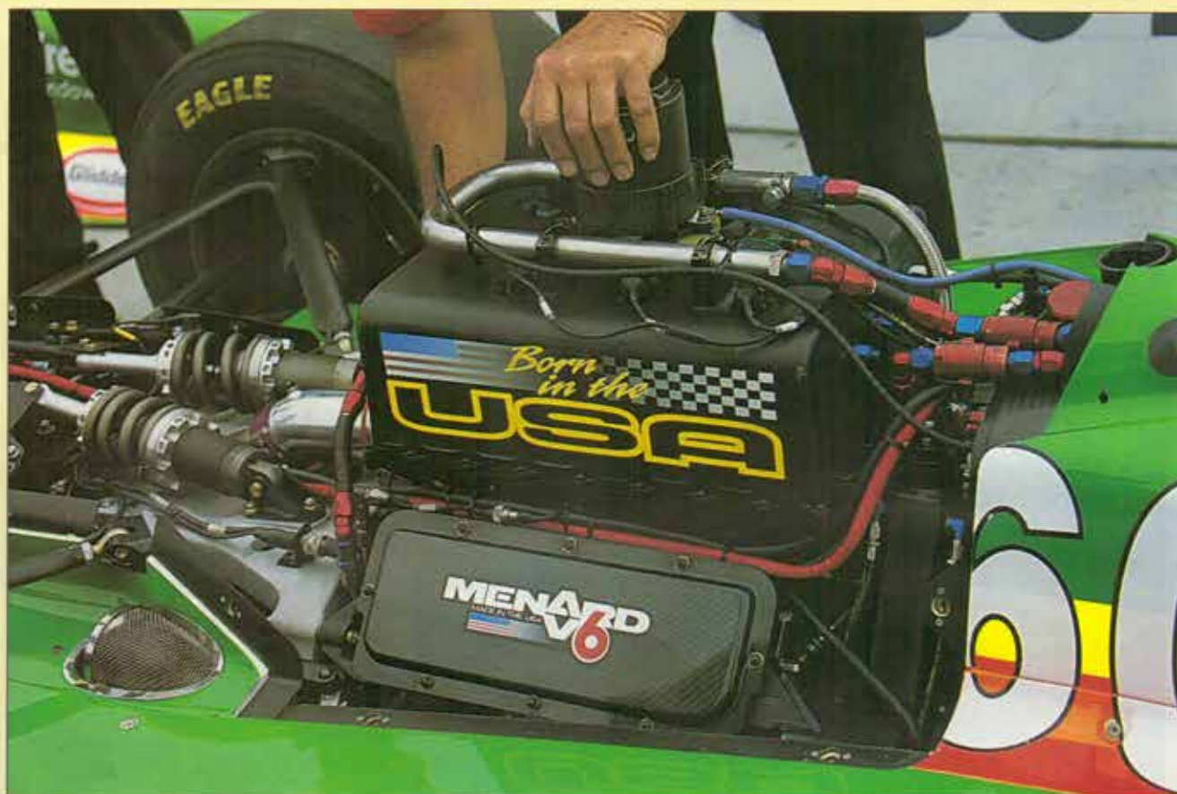
Team Menard, whose extensively developed stockblock Buick V6 now carries its name, secured a 1-2 in qualifying, with Scott Brayton on the pole.
